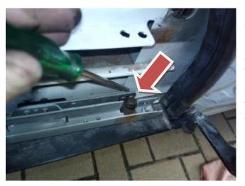
Now place the straight piece of track onto the door opening. The trick here is to NOT have the end where the mechanism that holds the door in the open position hard against the bus frame. Where my screwdriver is pointing make sure there is enough clearance for the stopper to move as the door roller pushes against it. About 10mm should do it. Before screwing it to the floor put the roller into the track and fully open the door.
