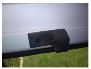
Remove the upper rubber stopper. We won't need this one, mainly because Ford in their wisdom did not include the captive nuts in the alternate position, and because it is impossible to access behind we will put in the too hard basket. It isn't really needed anyway.
