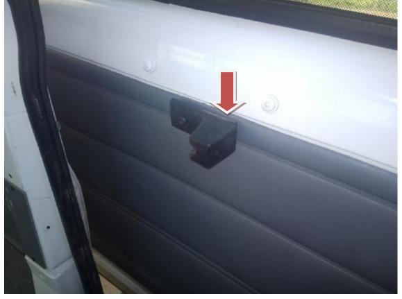
First job is to remove the rubber stops from the door.
