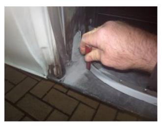
Place the track onto the floor upside down, making sure the track is hard up against the front of the step well where the plastic was trimmed in the previous instruction. Also make sure the track is hard up against the body work at the rear of the step well. Using a pencil, mark where it fits onto the floor of the step well. This step makes sure that the original shape is maintained when the track is modified later.
