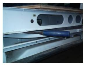
The spot welds that are under the floor need to be 'encouraged' out with some force. The best way is to use an old wood chisel and hammer and cut through the welds. They will cut through with moderate force easily enough. The same chisel can be used to convince any other belligerent welds that drilling does not quite release.
