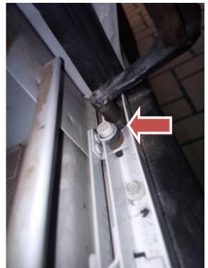
The stopper mechanism should be in the correct position without interfering with the door roller. Mark the position then screw in place at this end first, making sure there is nothing on the underside of the floor first. The front end of the track needs to be hard against the frame of the bus.
