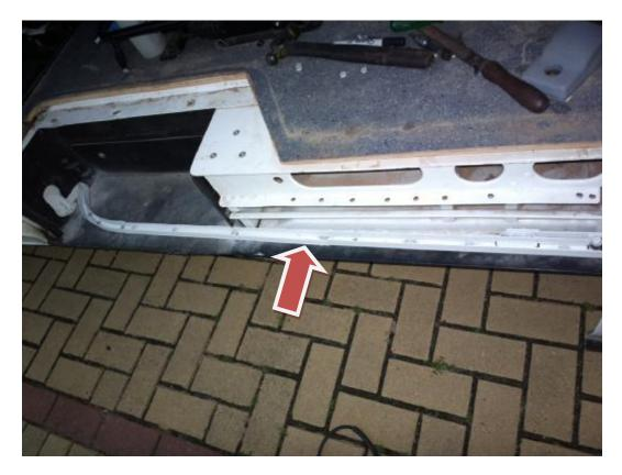
All that is now required is to cut a piece of U section to length. I only had a piece of box section that I cut the top from. Paint the track, I used white to make it look like part of the frame. One day I will remove and weld the two sections together, as I did not have a gas torch at the time.
