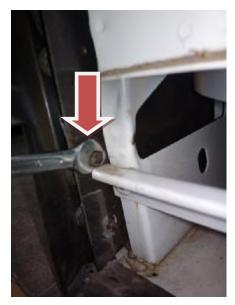
In removing the trim from the floor and step well there are two nuts on the back of the vertical trim closest to the rear of the bus. It is also glued on to the main trim. So don't half wreck it like I did trying to figure it out!
