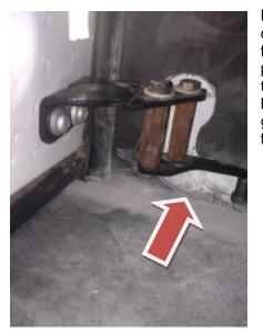
Bolt the roller into place on the door. Note it is upside down to the original position. Gently close the door as far as it will close. It won't close all the way as the plastic step well cover is in the way. Scribe out where the roller interferes with the closing action. I used a hole saw to cut a series of holes then a wood rasp to get the final fit so that the roller will allow the door to fully close.
