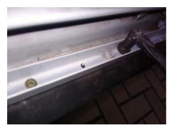
Screw the track to the floor, using the drilled spot weld holes. Then guide the roller into the track and check for clearance from the screw heads. You can see I used 8mm tek screws. Adjust the roller on the adjustment at the door end if required
