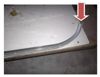
Next place the track onto something with a square corner. I have used a piece of scrap chipboard. This step is important as we will be wanting to replicate the closing action of the original track. Square up the long edge of the track along one edge of the square. Then mark with a pencil the outline of the track. Be accurate to mark the end of the curved part of the track.
