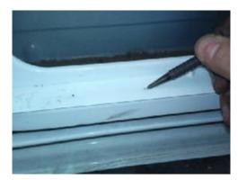
Now another tricky bit. We need to re-use the original track so we need to remove it from its original position. To do this requires drilling out the spot welds. Centre punch the middle of each spot weld, then using a small (say 3mm) drill, drill a pilot hole. Drill out each spot weld with an 8mm drill. You won't be able to drill out the spot welds underneath the floor, so brute force will be needed
